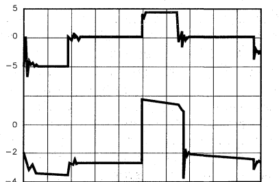
TIME BASE: 5µSEC/DIVISION UPPER TRACE: DRIVE TRANSFORMER SECONDARY LOWER TRACE: POWER TRANSISTOR BASE VOLTAGE
